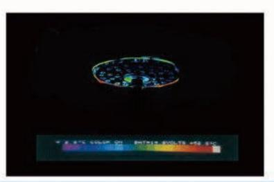
LED light source does not produce infrared, the temperature rise above surgeon's head is less than 2°C.
